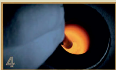
The gold is then melted and then weighed again. Post which, it is cooled and cleaned in deionized water
